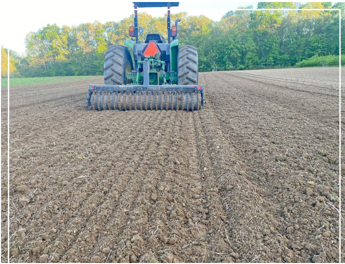
Figure 5. Cultipacking before planting, especially in fluffy soils, helps create a firm seedbed and prevents small-seeded species from being planted too deeply. After planting, cultipacking helps achieve ideal seed-to-soil contact to maximize germination rates.
