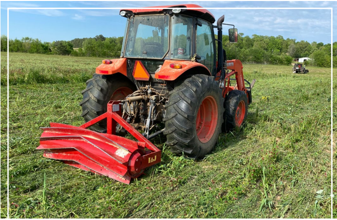
Figure 13. This regenerative cool-season plot was no-till drilled just before roller crimping. The roller crimper terminated a portion of the vegetation, creating a thatch layer at ground level to suppress weeds while the incoming warm-season planting establishes.
