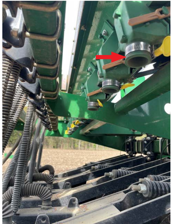
Figure 3. No-till drills are extremely versatile planting implements. No-till drills may be used to drill into the soil, top-sow into thatch, and top-sow into tilled seed beds. Top-sowing with a no-till drill distributes seed more precisely compared with spin-type spreaders. By unhooking the drop tubes when top-sowing, seeds are broadcast uniformly onto the soil surface, reducing available growing space for weeds to colonize.
